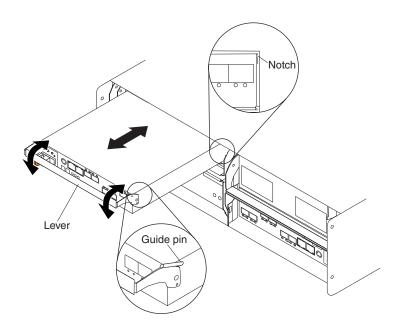
Figure 21. Removing and replacing a controller
